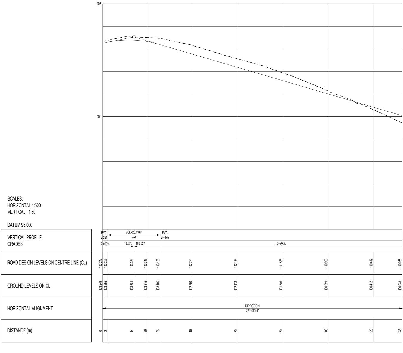
LONGSECTION ALIGNMENT ROAD 7 FROM 0.000 TO 132.750
