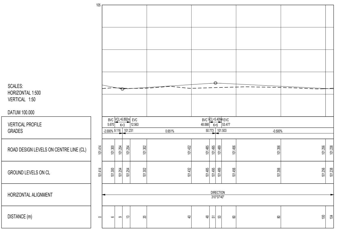
LONGSECTION ALIGNMENT ROAD 9 FROM 0.000 TO 103.616
